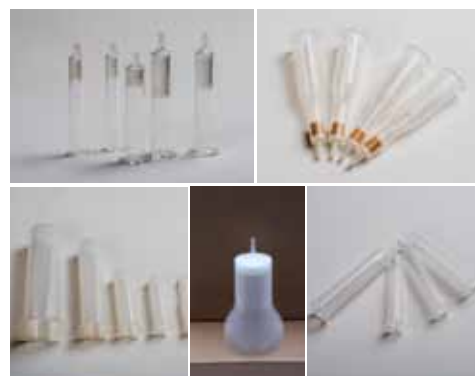
Figure 1 SPE Cartridge (General Cartridge, LRC, Glass Cartridge, LDC cartridge, Flangeless Cartridge)
