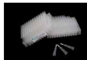
Figure 3 Integrated micro SPE plates
